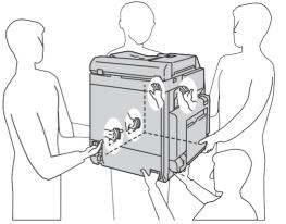
Locate this product on a level and sturdy surface that can withstand a weight of 68 kg (minimum configuration). Otherwise, if tilted, the product may fall over and cause injuries.
